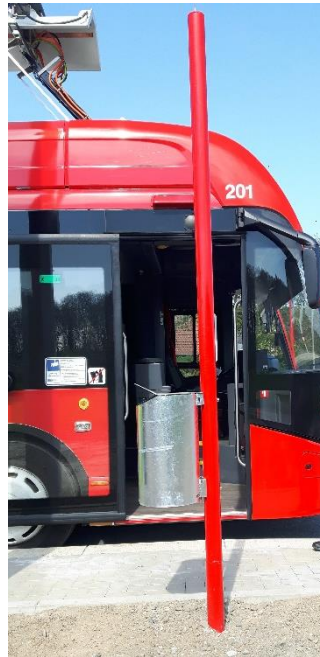
Figure 8. Proposed method for bus positioning guidance for drivers in ASSURED
