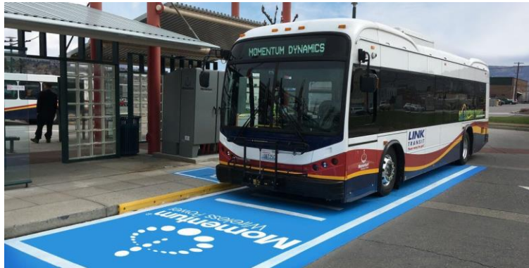
Figure 11. Static inductive charging (Lambert, 2018)
