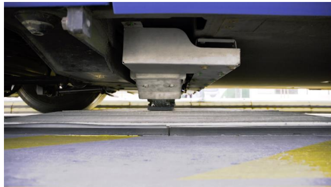
Figure 5. Ground-based ACD (Alstom SRS)
