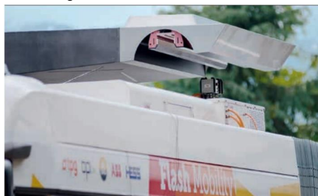
Figure 9. TOSA charging system (Hitachi-ABB)
