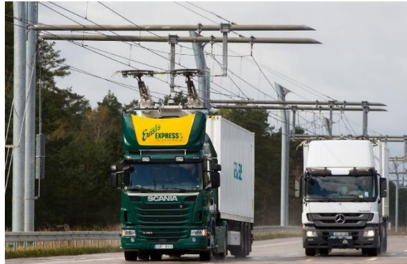
Figure 6. Catenary charging of hybrid trucks (picture: Scania)
