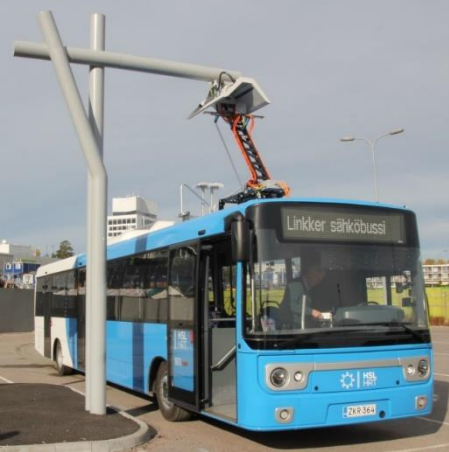
Figure 3. Roof-mounted ACD (Photo: VTT)
