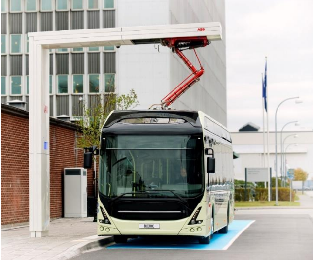
Figure 2. Infrastructure mounted ACD (ABB)
