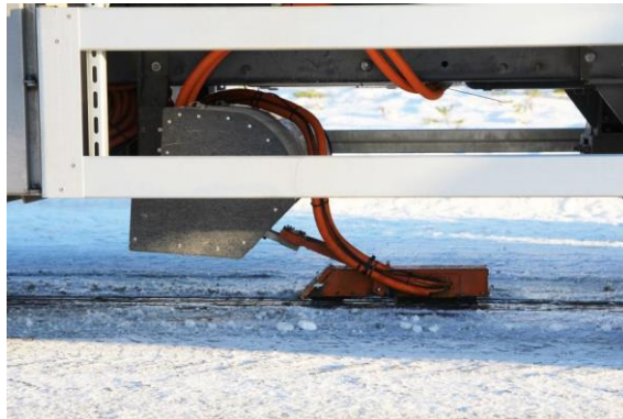
Figure 7. Underneath dynamic charging (Ravenscroft, 2018)
